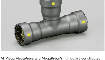
All Viega MegaPress and MegaPressG fittings are constructed with the patented Smart Connect feature. The Smart Connect feature is a quick and easy way for installers to identify connections that need to be pressed. Testing for leaks using the Smart Connect feature is not a replacement for testing to the requirements of local codes or standards.
